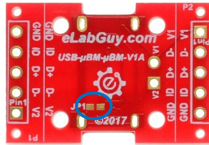
Figure 6: PCB back with optional Jumper connects Shield to GND
