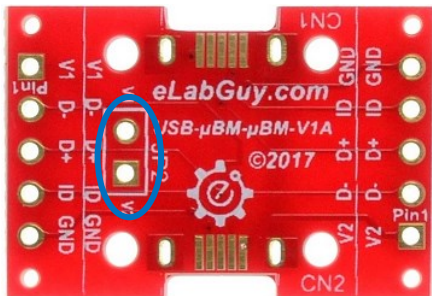
Figure 5: PCB front with open circuit on VCC pin in series
